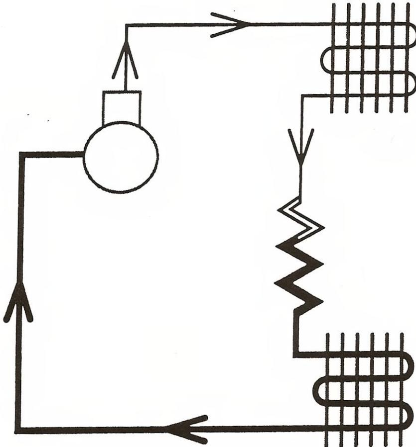
You really can't make it much simpler than this. That's the compressor shown up there at the left. When refrigerant leaves the compressor (follow the arrows) it goes into the condenser, then on through a component called the metering device... more on that shortly....then on to the evaporator. Then the refrigerant heads back to the compressor, then back to the condenser, then.... Well, you get the idea.
